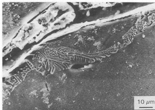
Figure 3 SEM micrograph of intermetallics present at the mould-casting interface.
